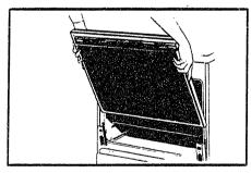
To REMOVE door, open to BROIL position, or where you feel hinge catch slightly. Grasp door at sides; lift door up and away from hinges.
